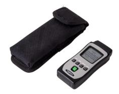
The TIS PV1 Solar Power Meter is used to measure Solar Power. With this unit you can measure the optimal incident angle for Solar Panels & determine the best choice of Solar Panel. Measurements are displayed in W/M squared or BTU.
