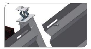
• When the last backing plate is reached, a hole of  $\emptyset$  5.5 mm should be bored, and the screw provided screwed into the slot and the hole created.
