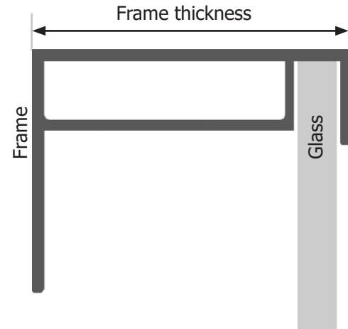
If frame thickness is  $\leq 35mm$  (1.4in), install with the TS4 label facing the PV module.
